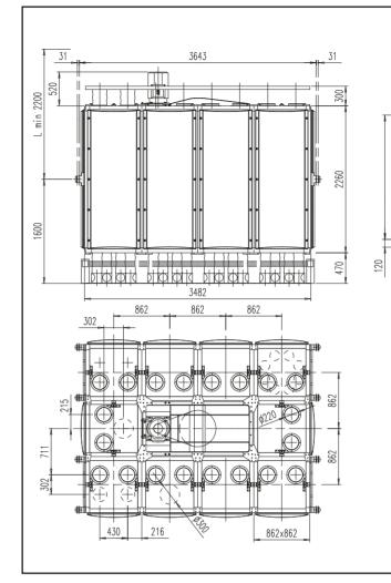
Sieve dimension = 740x740mm Net sieve surface =  $0,41 \text{ mm}^2$
