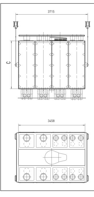
Sieve dimension = 740x740mm Net sieve surface = 0,41 mm<sup>2</sup>
