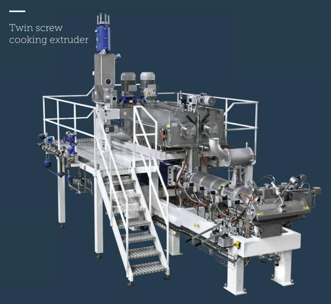
The TT cooking-extruder continuously and automatically gelatinizes flours and starches.
