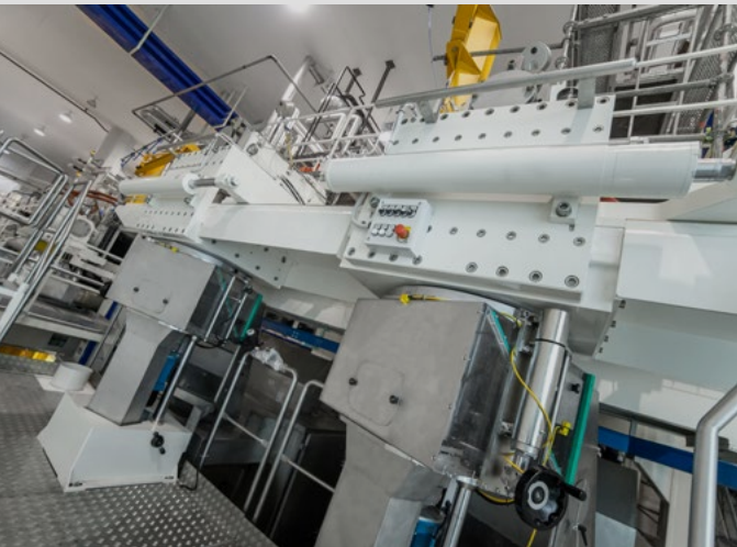
Pennaut 2T installed in a 6 t/h short-cut dry pasta line
